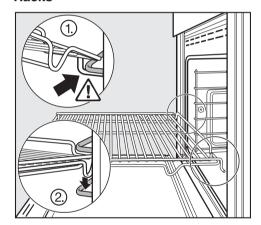
The racks are fitted with non-tip safety notches which prevent them being pulled right out when they only need to be partially pulled out.
